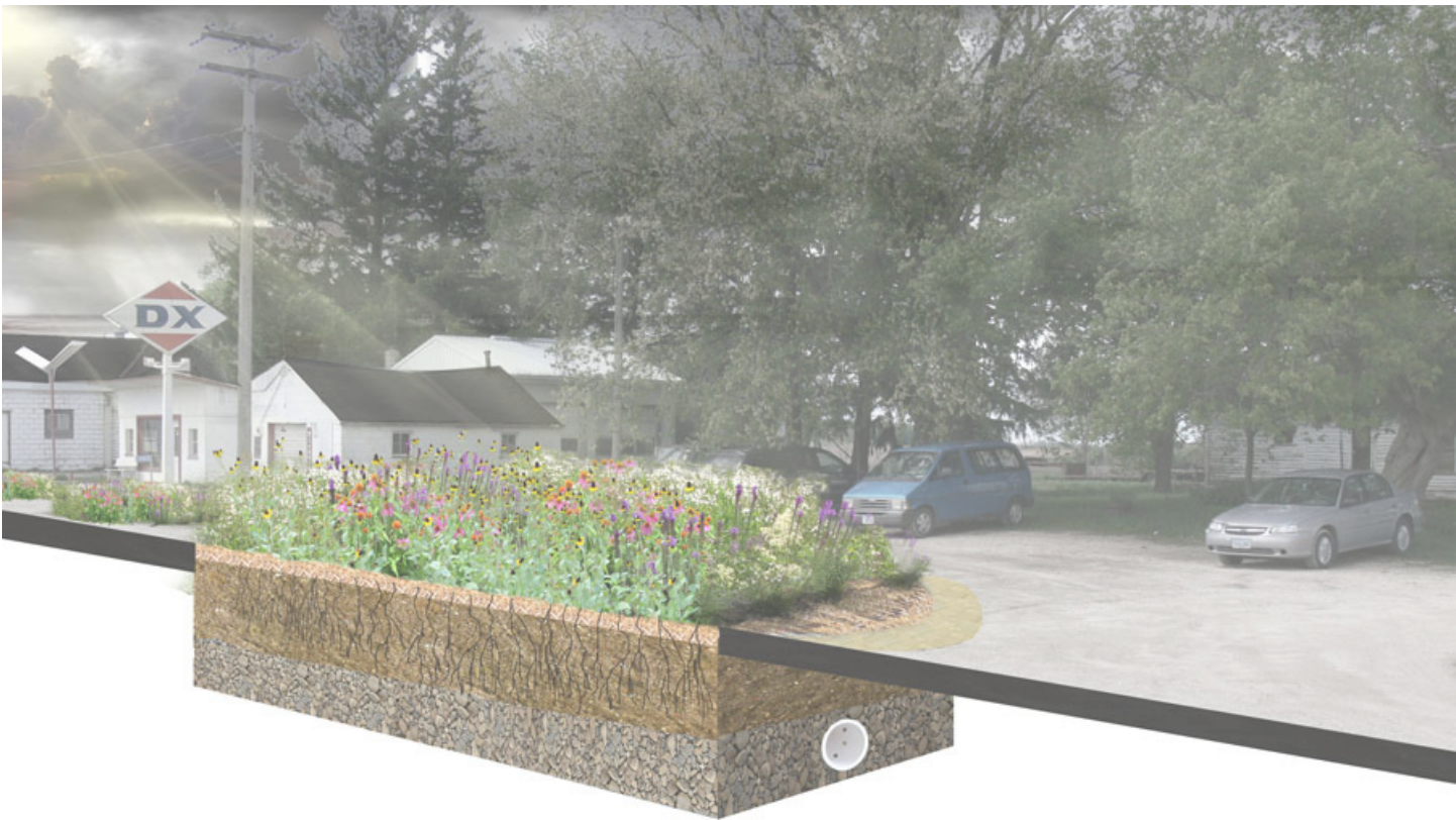
Above: A rain garden in the auxiliary parking lot of the Irish Shanti restaurant would help capture, filter, and infiltrate runoff to reduce flooding.
